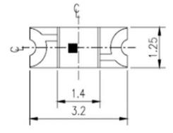
Note: 1. All dimension are in mm tolerance is  $\pm 0.1 \text{mm}$  unless otherwise noted.
